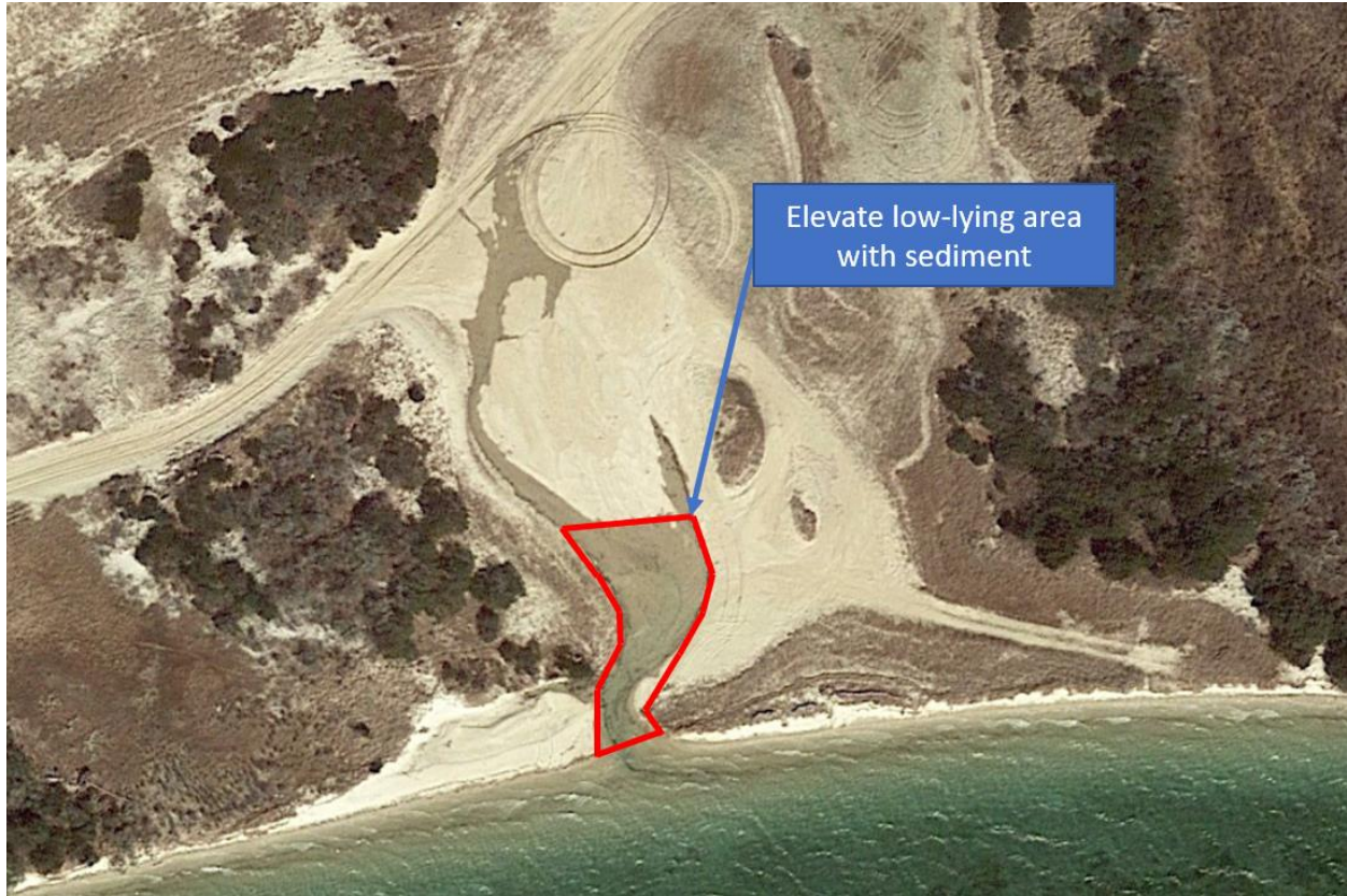
Figure 107. Conceptual footprint for elevation with import at 1 st and 2 nd Point – February 2018 Aerial
